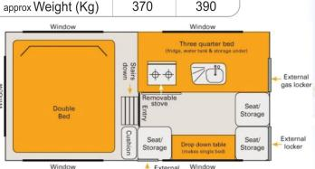
The dual cab Trayon Camper sleeps as many as you can fit into your ute (4-5). The bench with fridge and storage underneath can
